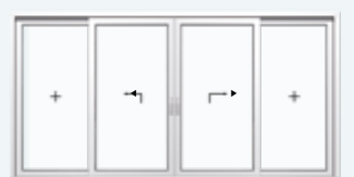
System C 2 lift/sliding sashes, 2 fixed panes
